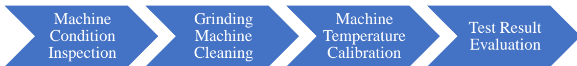
Figure 5. Stages of Grinding Machine Maintenance and Calibration Activities
